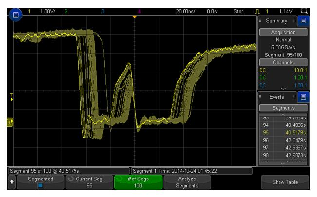
Figure 13a. Screen showing an overlay of all 100 segments for worst case waveform analysis.
