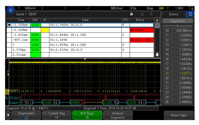
Figure 20. Segmented memory being used in conjunction with SENT bus serial decode resulting in maximum insight to the serial bus.
