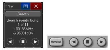
Close-up on buttons on the front panel of the scope. Alternatively, you also can use the touch navigation control.
