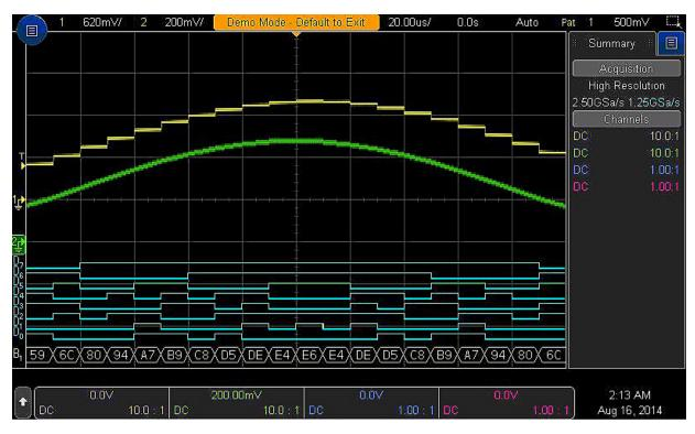
Figure 22. Optional digital channels allow a timing view of up to 16 channels. Tightly integrated, they work with the analog triggers and serial triggers/decoding.
