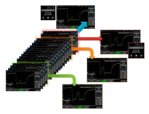
Figure 13. Segmented memory reveals different types of glitches are taking place.
