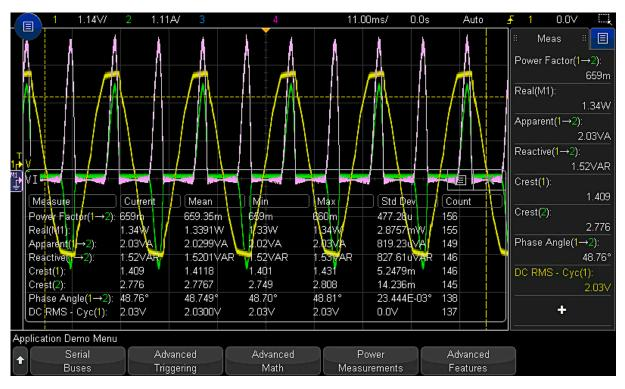
Figure 28a. Integrated power measurements make quick work of analyzing power producing and power consuming devices.
