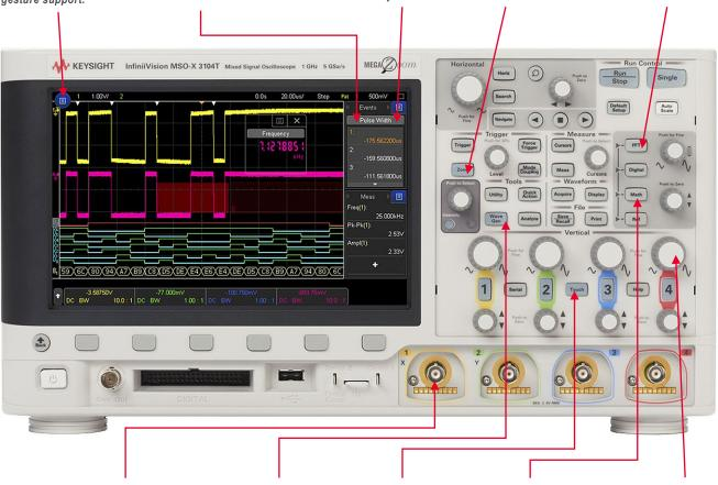
**AutoProbe** interface supports various active, differential, and current probes.
