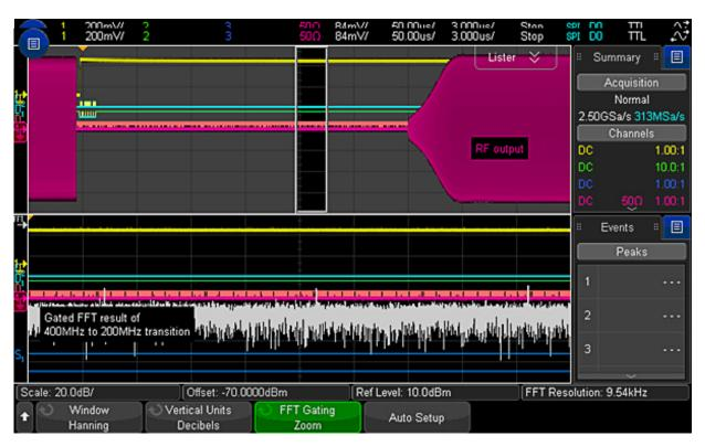
Figure 21a. Triggered on a SPI command, the RF signal is still at 400 MHz as indicated in the frequency peak search result lister.
