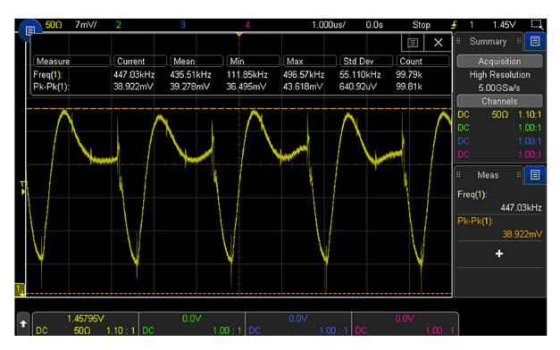
Figure 29b. 3000T X-Series and N7020A acquire not only the power rail ripples but the high frequency transients as well.
