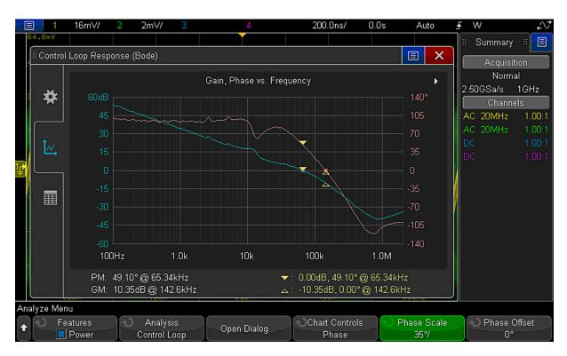
Figure 28b. New control loop response analysis (bode plot) shows the gain/phase plot over frequency sweep.
