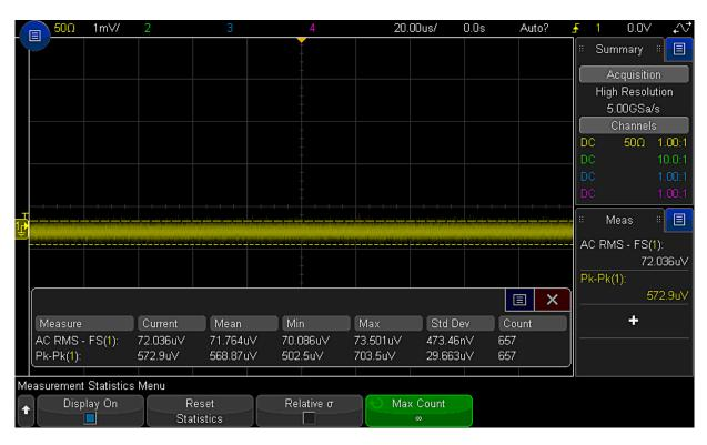
Figure 12. High resolution mode allows you to lower your noise and increase your resolution up to 12-bits.
