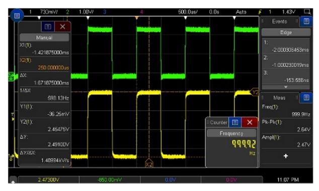
Figure 3. Side bar with movable docks allows information to be placed on the screen precisely where you want it for documentation.
