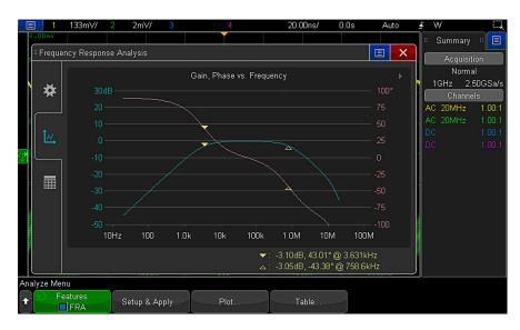
Figure 23. Frequency response analysis plot (Bode gain & phase) of a bandpass filter.
