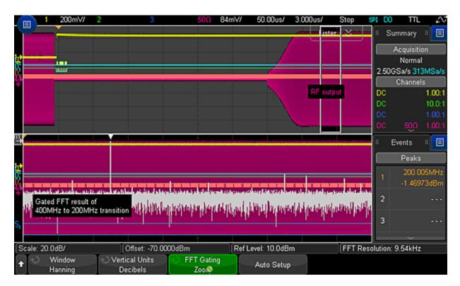
Figure 21d. RF signal settled down at 200 MH as indicated in the search lister.
