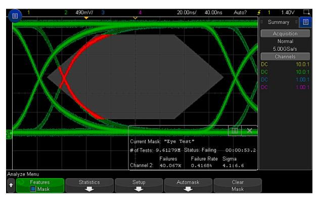
Figure 27. Hardware accelerated mask testing allows testing against a golden waveform or user created mask to find violations. In this example we captured over 5M tests in only 30 seconds.
